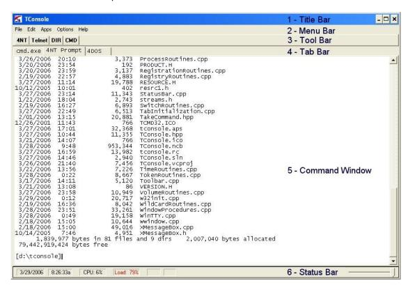
1. The **Title Bar** is the same as the one used in most Windows applications, with a control menu button on the left and the minimize, maximize, and close buttons on the right. You can adjust the size of the **TCI** window using standard window techniques, but see Resizing the TCI
